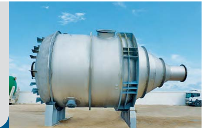
Flash chamber with Alloy 28
